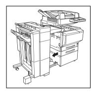
2 If finisher F-8430 is installed, open right-side door FN7.
